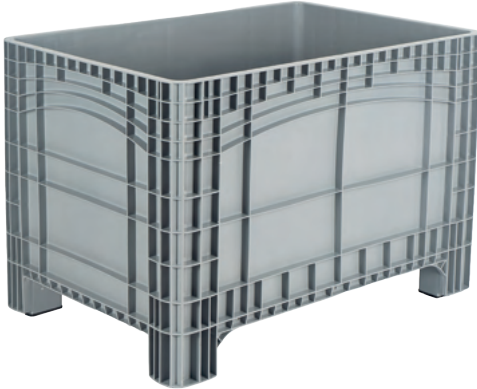
K-550 En/W Boy/L Yüksek/H Hacim Dynamic Static Dış / Ext 800 x 1200 x 800 mm Volume Capacity Capacity İç / Int 732 x 1106 x 617 mm 500 Lt 400 Kg 2500 Kg Kapalı / Closed Ağırlık / Weight 22,00 kg
